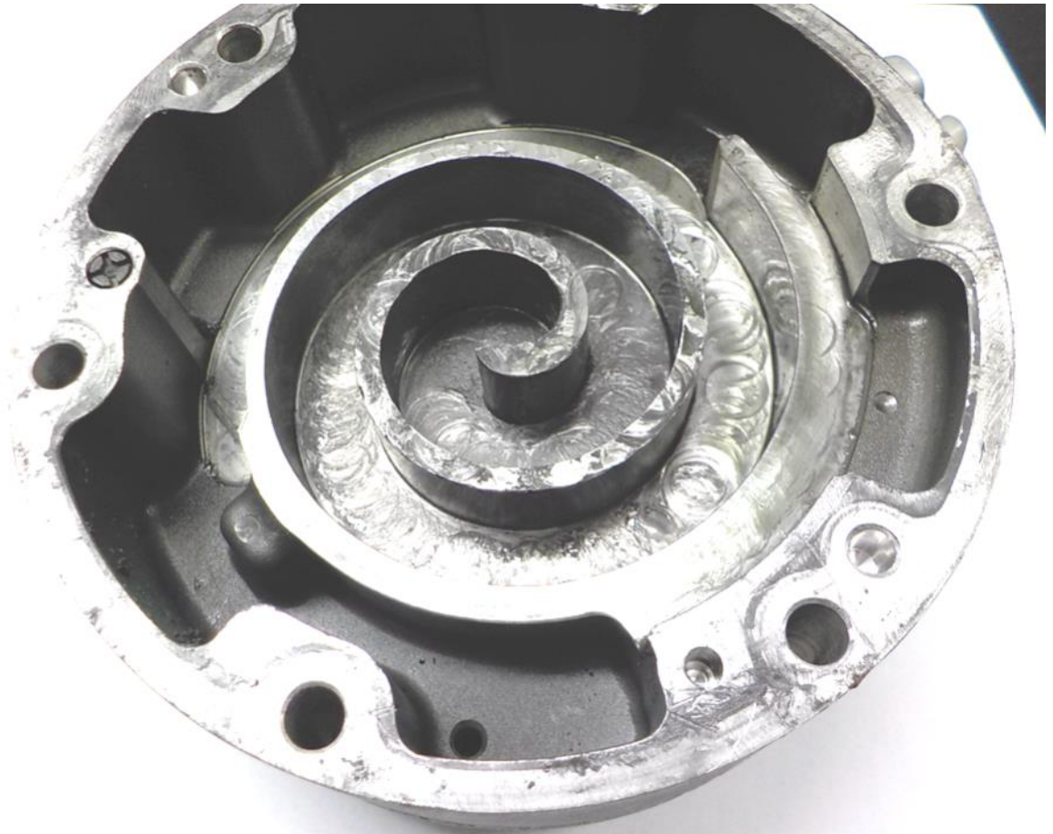
The static scroll of the compressor
